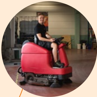
A scrubber using recycled water from the washing process of turned components.
